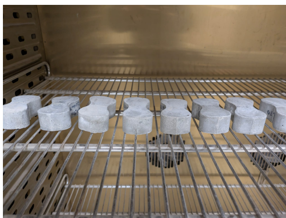
Figure 7. Fe-SMA briquette specimens placed inside the laboratory chamber prior to thermal treatment.
