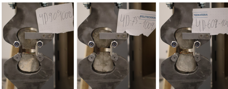
Figure 9. Specimens during pull-out testing at inclination angles of (left) 90°, (center) 75°, and (right) 60°.
