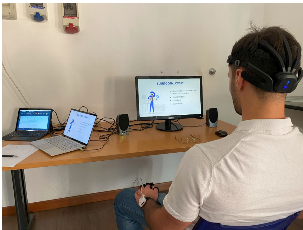
Figure 1. Experimental settings. The participant sat in front of the PC to provide learning materials and wearing the EEG, PPG, and EDA signals collection equipment.
