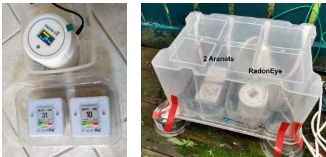
Figure 1. Parallel measurements with two Aranets and one RadonEye indoors (left) and outdoors. In outdoor operation, two further layers of plastic sheets are added to protect against weather and the compound was fixed to the balcony grid with the green string visible in the back. The white cables serve for power supply of the RadonEye and for dose rate monitors operating in a similar box nearby (not shown). After a few days the Aranets were moved to a similar housing about 2 m away.
