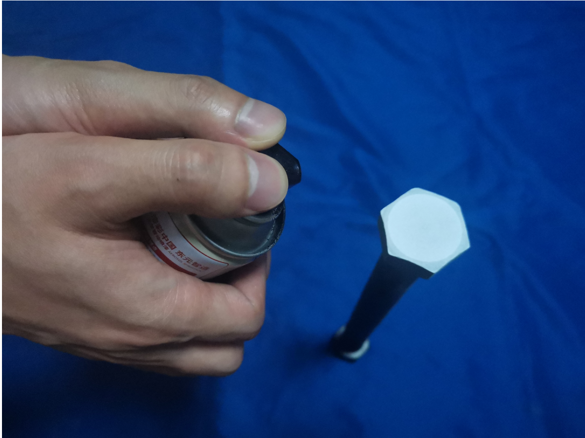
Figure 2. Method for spraying speckle patterns on the bolt head surface.
