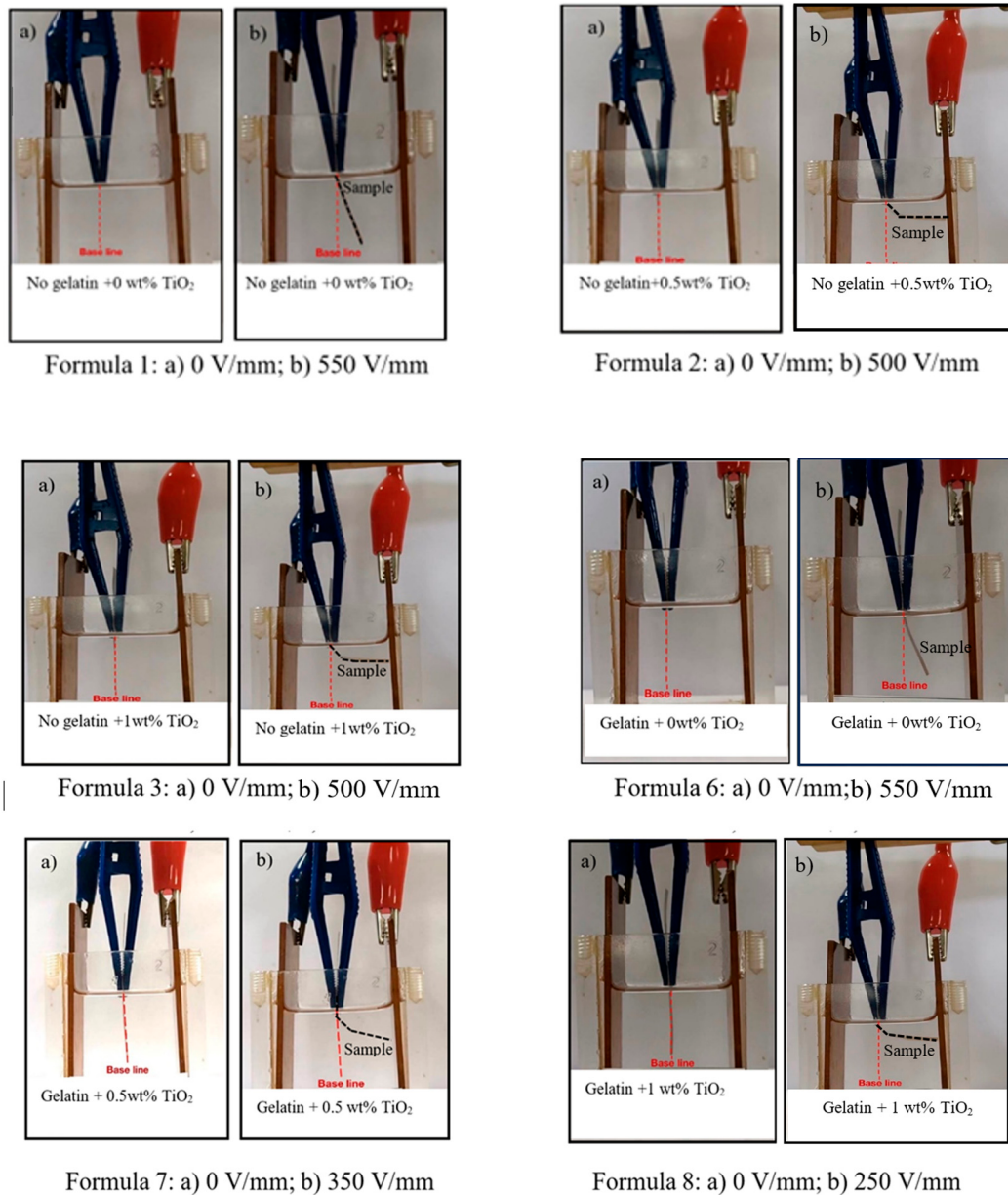
Figure 10. Electromechanical response of Formulas 1, 2, 3, 6, 7, and 8 in bio-chitosan composite films, measured from 0 V/mm to 550 V/mm: a) at 0 V/mm and b) at the onset of electromechanical response. Note: Formulas 4, 5, 9, and 10 did not exhibit an electroactive response due to excess TiO 2 , causing brittleness and cracking.
