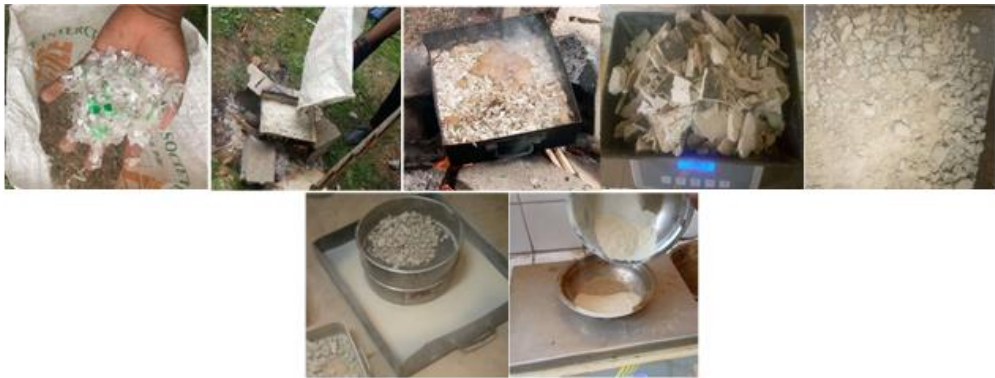
Figure 2. Artisanal micronization process of PET bottles.
