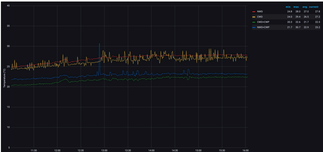
Figure 7. The dashboard displays root-zone temperatures in different cooling treatments.
