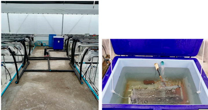
Figure 2. Cooling water tank system to generate 10-15 °C cold water.
