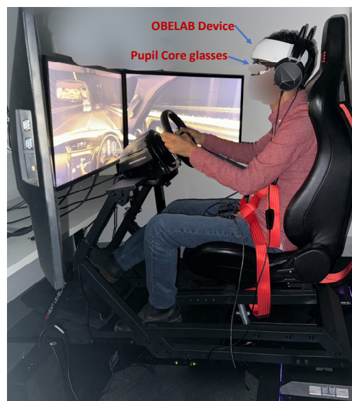
Figure 1. Driving simulator setup designed to replicate real-world vehicle dynamics and driving conditions using motion platforms and responsive control hardware.
