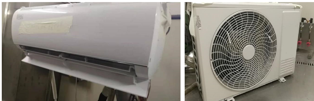
Figure 3. Photographs of the R32 prototype AC unit.
