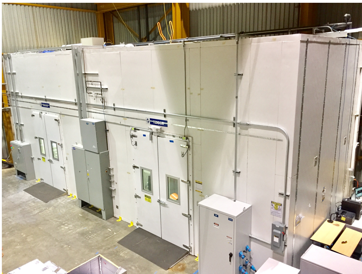
Figure 4. A Photograph of LBNL's psychrometric test chamber.
