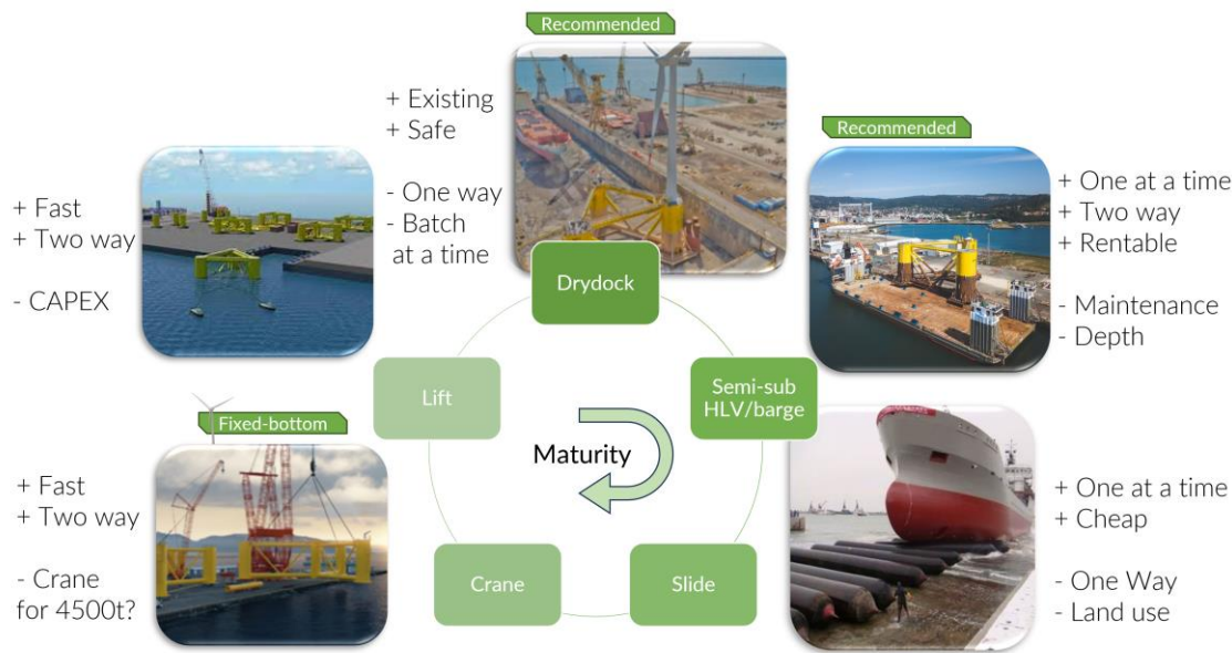
Figure 3.1. Ways to launch a floater. Pictures courtesy of: Principle Power, Ocergy, Bardex.
