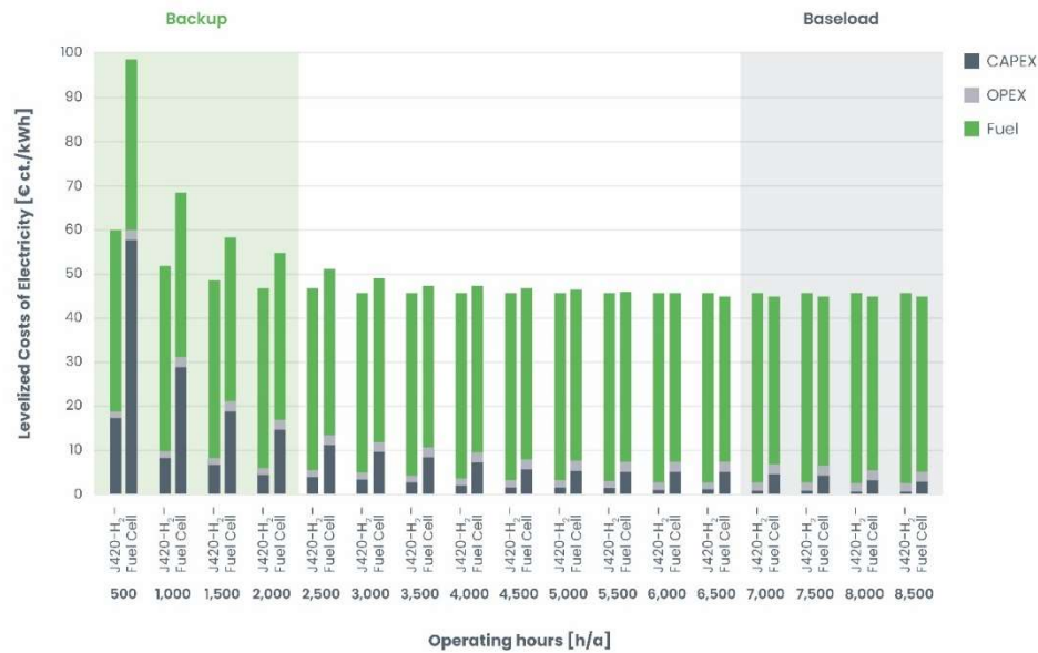
Figure 7. LCOE for H 2 -Engines and H 2 -Fuel cells.
