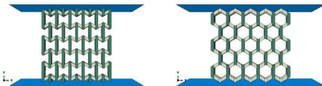
Figure 10. FEM models of re-entrant and hexagonal cellular structures and their reinforcement locations (green - reinforcement, gray - nylon) [17].
