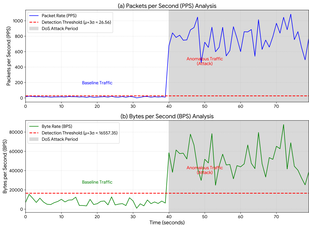
Figure 4. DoS Attack Detection Using PPS and BPS Metrics. Detection of a DoS attack (shaded region, t \geq 40 s) through data-rate monitoring. A baseline statistical threshold (red dashed line), corresponding to \mu + 3\sigma , was established based on normal operation ( t < 40 s). Upon attack initiation at t = 40 s, both (a) Packets per Second (PPS) and (b) Bytes per Second (BPS) exhibit immediate and significant spikes that exceed the threshold, validating the method’s effectiveness in identifying high-volume attacks.
