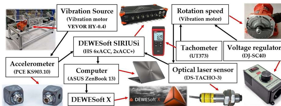
Figure 7. Measurement chain for detecting and recording vibrations generated by rotating eccentric weights on laboratory equipment.
