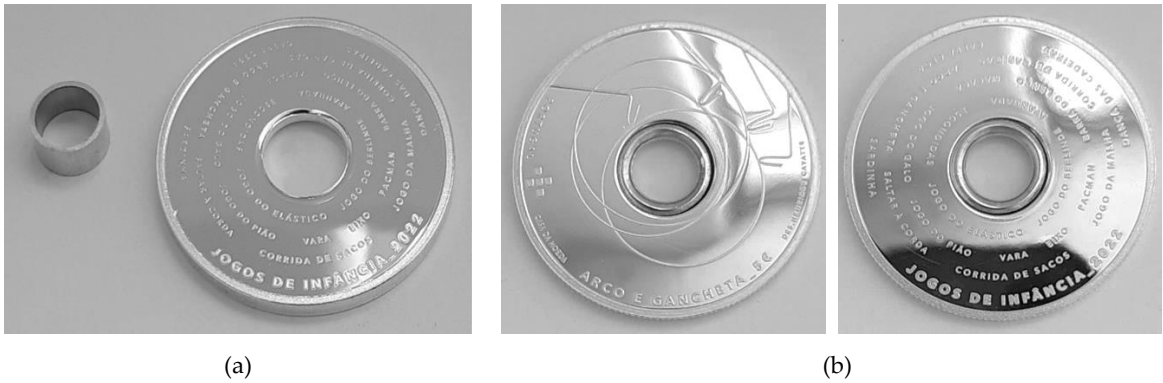
Figure 12. (a) Preforms and (b) manufactured coin with a rotating element of C-shape section.
