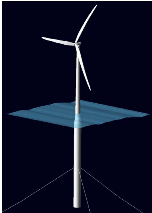
Figure 1. Sketch of the NREL 5-MW wind turbine on the OC3-Hywind spar. Source: Jonkman and Musial [17]
