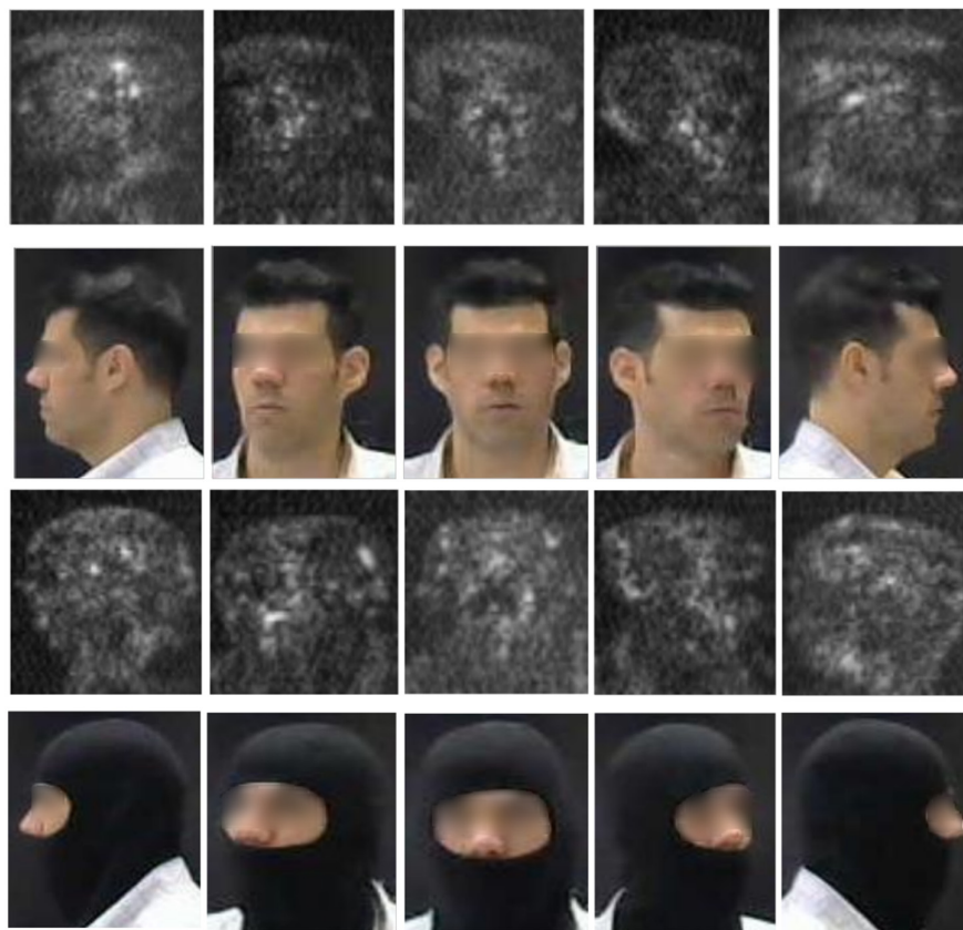
Figure 1. Unconcealed THz images of subject ID #10 across five distinct facial postures, and their visual counterparts. The top two rows present THz unconcealed faces across all facial postures with their corresponding visible images below, while the bottom two rows present the THz concealed faces across all facial postures with their corresponding visible images below. The THz samples demonstrate the inherent challenges of the active 340 GHz modality, characterized by low spatial resolution, high acquisition noise, and sparse geometric representations that obscure fine-grained facial biometrics.
