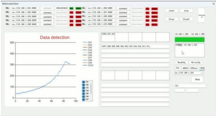
Figure 22. Normal working condition of parachute cords tension acquisition system.
