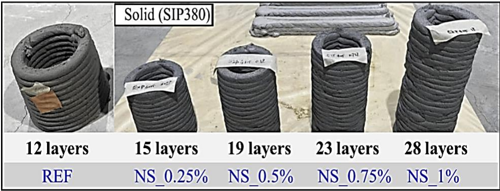
Figure 11. Buildability of printed elements with increasing NS content. Modified from [117].
