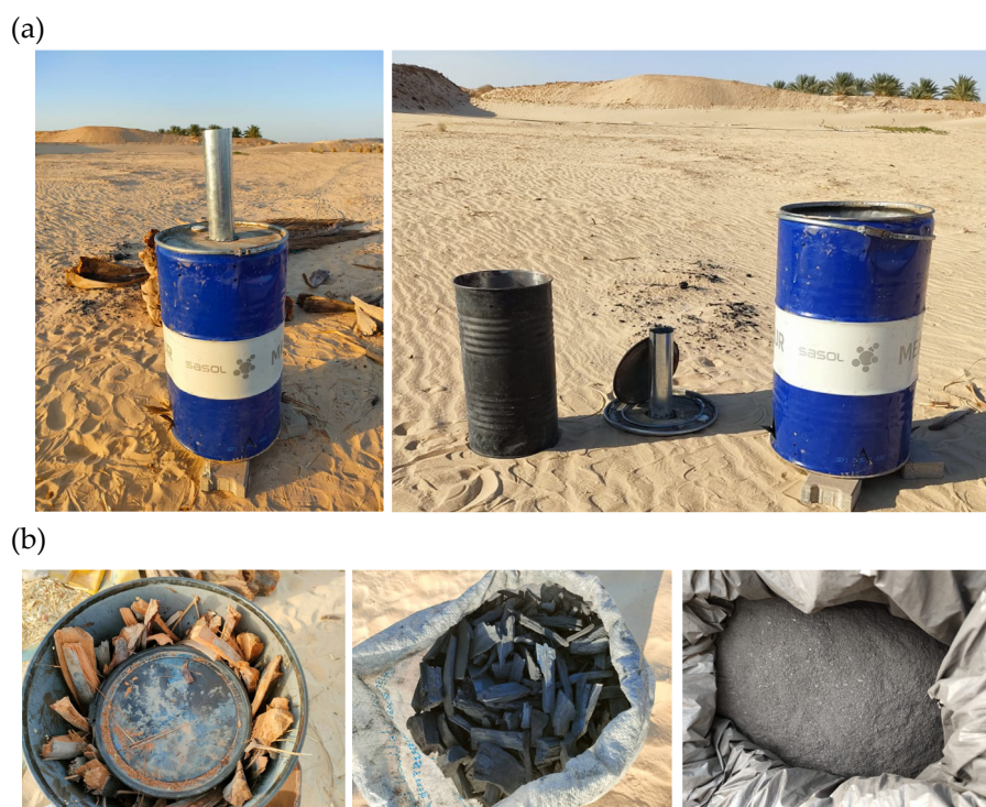
Figure 1. Palm, potato, and maize biochar preparation. (a) The double-barrel pyrolysis unit; (b) The biochar produced using a double-barrel pyrolysis unit.
