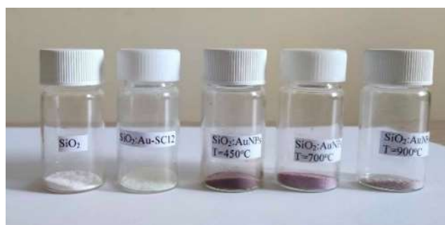
Figure 1. Preparation scheme for SiO 2 :AuNPs at heating, starting from SiO 2 :AuSC 12 H 25 and photographs of the obtained ceramic pigments.
