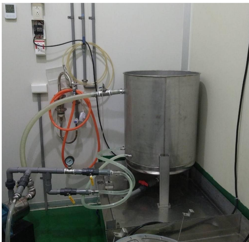
Figure 2. The 250-L device: (A) 250-L stainless tank, (B) water outflow pipe, (C) gas intake, (D) motors, (E1 and E2) water inflow pipes, (F) the drain to release water and collect seeds. The blue arrows indicate the direction of water.
