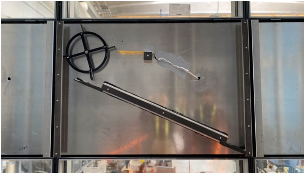
Figure 11. The PE-EHS cantilever, configured within the wheel setup, is installed in the façade within a laboratory testing facility. The airflow within the cavity triggers the rotation of the wheel, and the magnets positioned at its extremities generate a magnetic force with the magnet located at the end of the PE cantilever, thereby enabling vibration.
