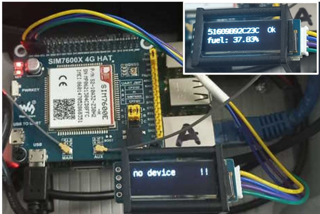
Figure 16. IoT Gateway and IoT platform: IoT gateway with led screens device reading and data communication to the IoT platform to the IoT platform.
