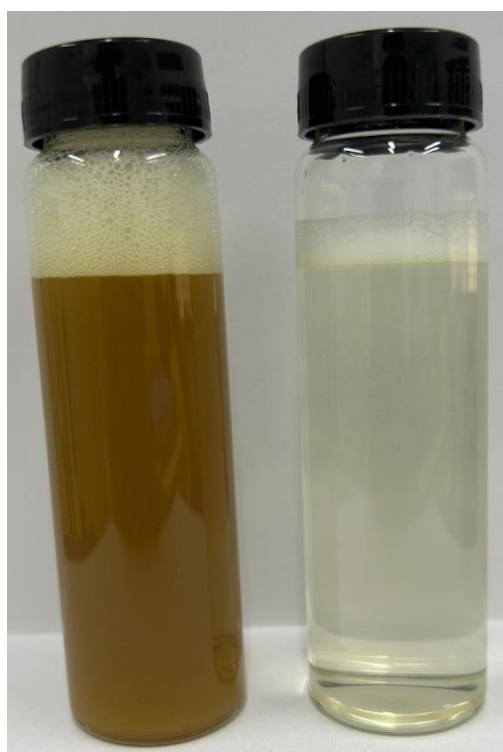
Figure 21. Synthetic oily effluent before and after filtration with the BC membrane.
