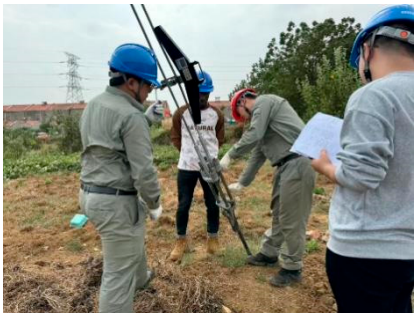
Figure 1. On-site Measurement of Tension Forces.
