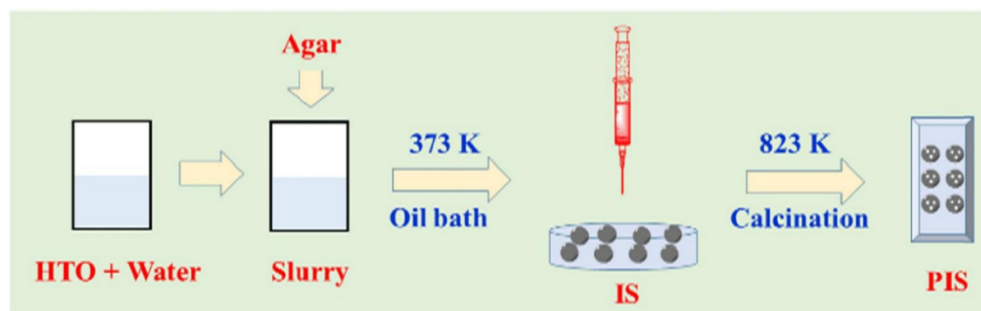
Figure 24. Schematic diagram of the synthesis of titanium-based ion sieves (ISs) and porous ion sieves (PISs). (Reproduced from [79] with permission).
