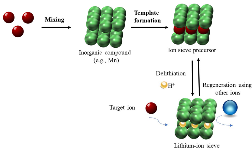
Scheme 1. Schematic representation of the preparation process for lithium ion-sieves.
