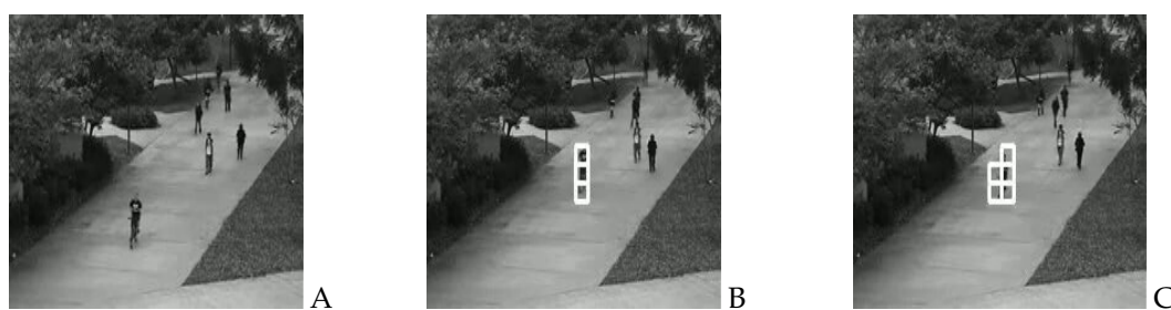
Figure 13. Abnormal behavior is marked with a white box. A. Normal video frame. B. Abnormal behavior detection with white box at time t . C. Abnormal behavior detection with white box at time t + 1 .
