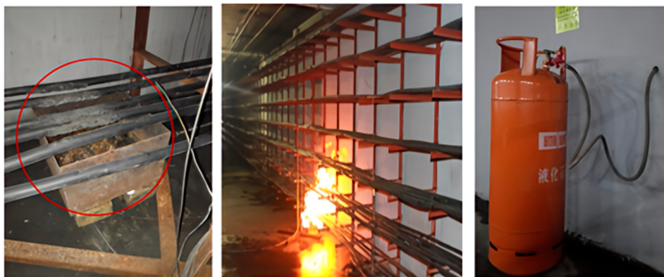
Figure 3. Fire source layout and propane burner.
