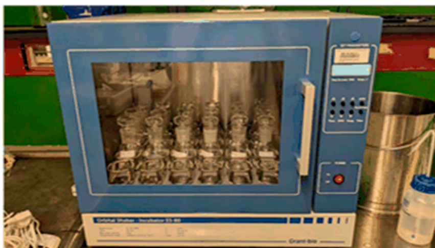
Figure 3. Batch adsorption separation of HTL of Lignin Products in the thermostatic oscillator.
