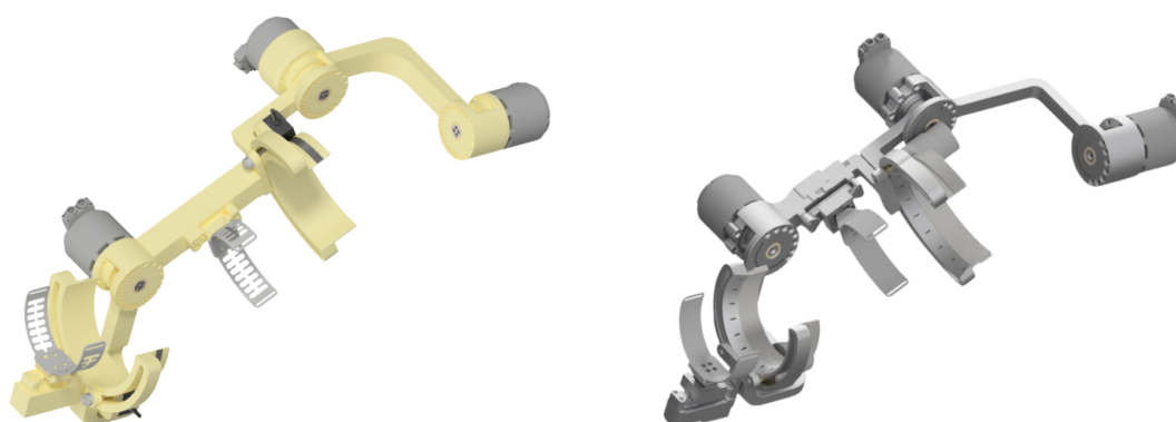
Figure A38. Comparison of initial design (left) and post-optimization cycle design (right) of the exoskeleton.
