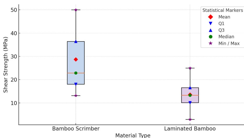
Figure 8. Plot of longitudinal shear strength for bamboo scrimber and laminated bamboo.
