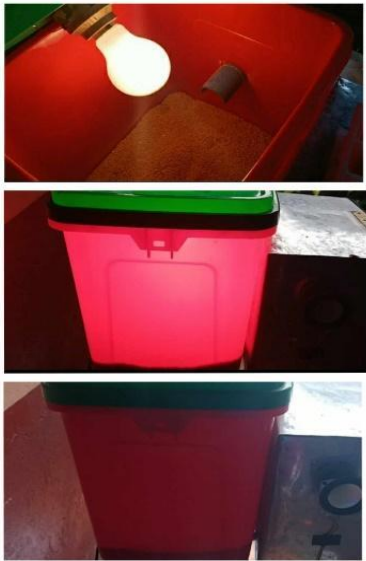
Figure 1. (Based on the respective pictures) 1. A) Temperature is less than 28°C, the lLamp bulb will turn ON. 2. B) Temperature is less than 28°C, the lamp bulb will turn ON (Outside view). 3. c) Temperature is greater than or equal to 33°C, the lamp bulb will turn OFF.
