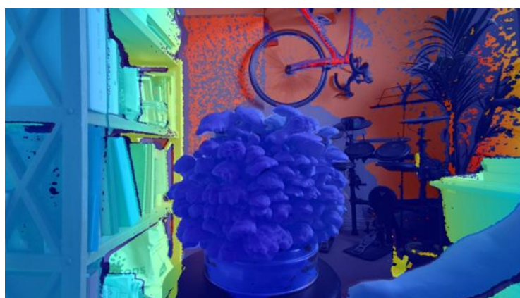
Figure 7. The result of blending the RGB and Depth images to check for alignment.
