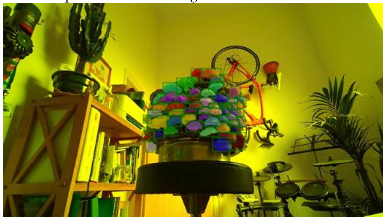
Figure 10. Detectron 2 Mask R-CNN inference on an RG-D image.
