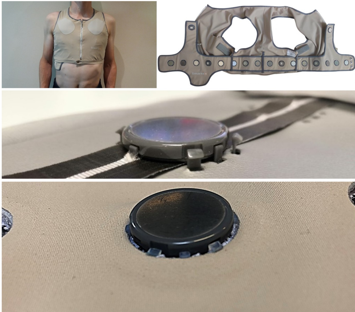
Figure 18. Top row: ASIC sensor harness worn (left) and open (right), exposing the sensors and the electrodes on the sensors and two textile electrodes. Middle row: ASIC sensor clamped to a 3D knit on two electrically conductive tracks, realized as conductive tapes (black). Bottom row: the belt textile with the reinforcement ring (seen as a slight bump in the photo) added on top of the conductive tapes.
