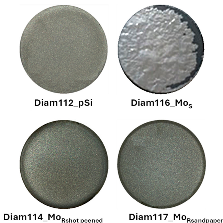
Figure 9. Photos of the diamond films deposited on p -Si and Mo substrates after 5 days of exposure in air (constant ambient temperature of 22 °C with stable humidity levels of about 65%).
