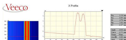
Figure 5. Measurement of the cross-section of the nickel line with a profilometer.
