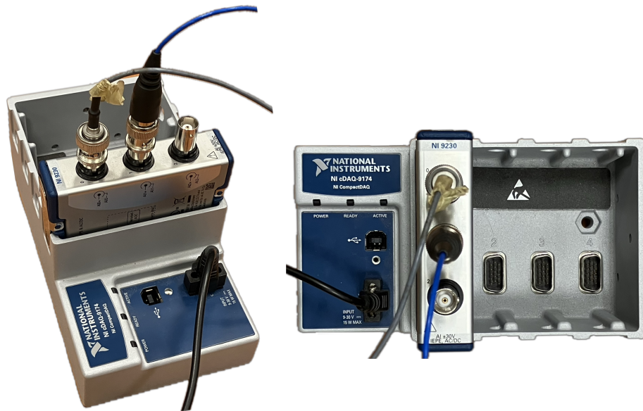
Figure 34. Data acquisition: NI cDAQ-9174 & NI 9230
