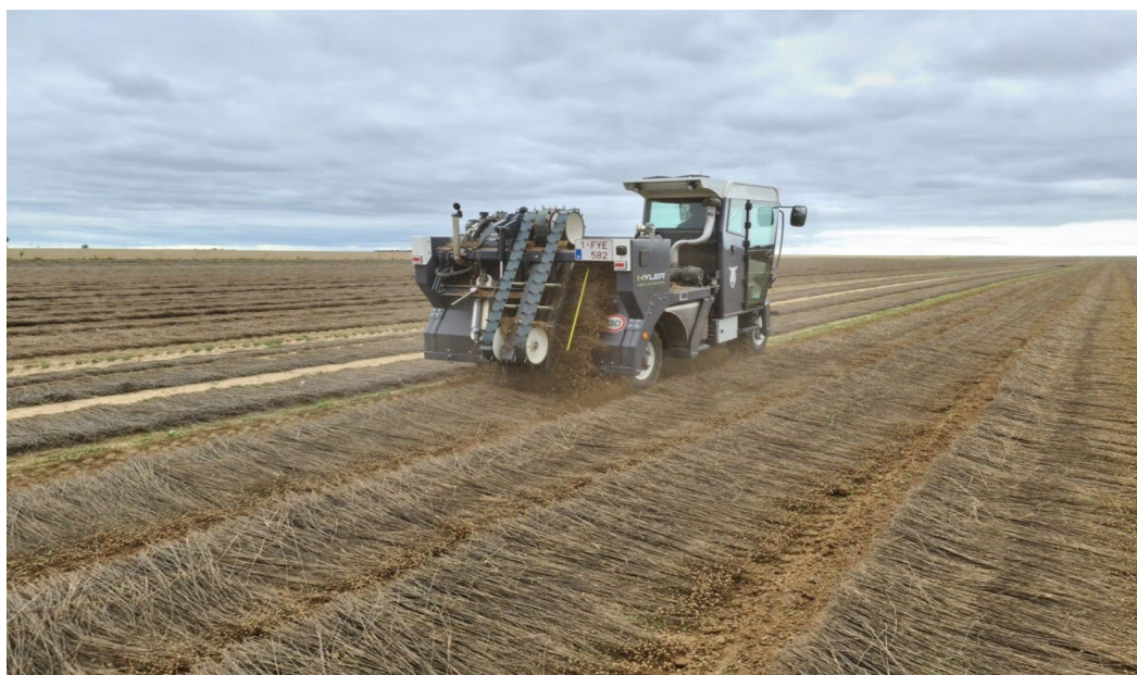
Figure 6. Hyler Easy-Turn 113A flax and hemp turner (Hyler, Meulebeke, Belgium) in operation.
