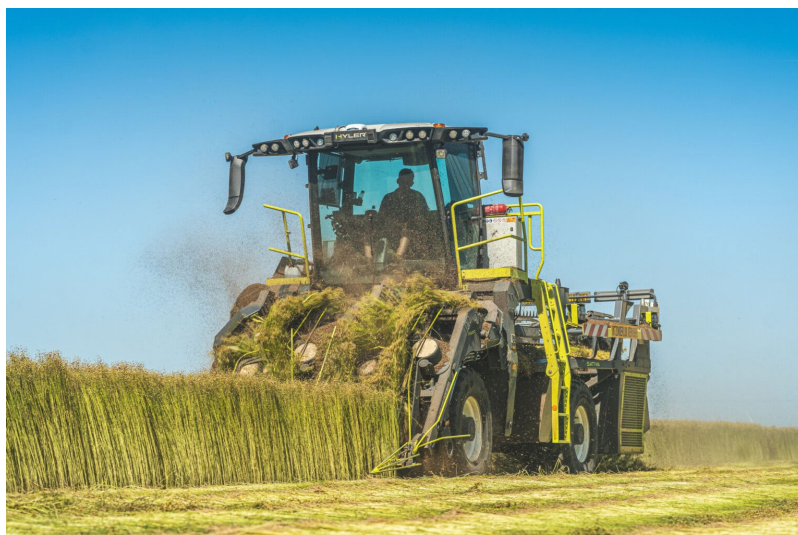
Figure 4. Sativa FS40 harvester for harvesting flax (Hyler company, 8760 Meulebeke, Belgium).
