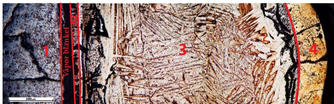
Figure 9. Change of microstructure along the cross-section of the \text{CaTiO}_3 sample / Grade 2 alloy after isothermal interaction at 1720 °C for 430 s.
