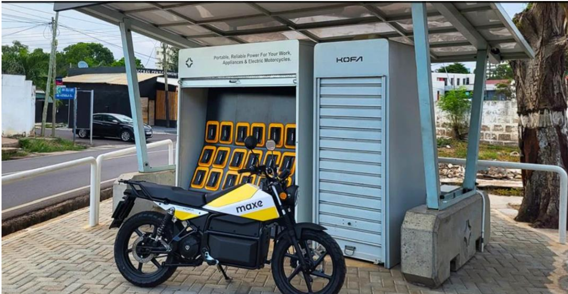
Figure 2. Battery swapping station for electric motorcycles in Africa. The KOFA-branded kiosk holds an array of swappable battery packs; riders dock their depleted unit and retrieve a charged one in minutes, reducing downtime while supporting a managed lifecycle. Source: https://www.tycorun.com/blogs/news/top-10-battery-swap-station-companies-in-africa?srltid=AfmBOoqtOXjmLvjnW5dI57wGVP_Wt2t2OWw5JCu2Ktn6eMaXdz7mdJIK .
