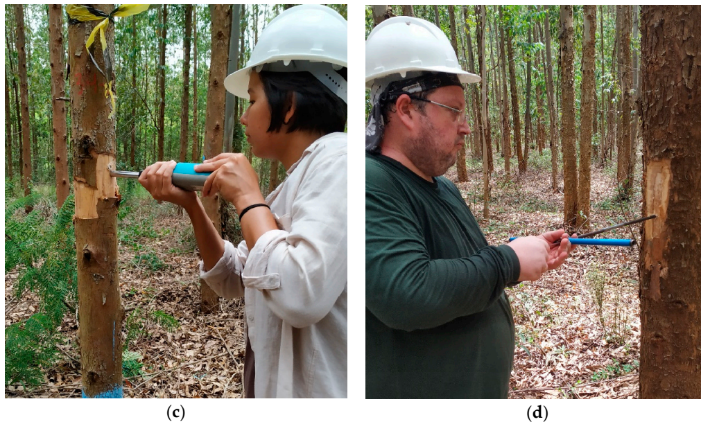
Figure 1. Ultrasonic wave propagation test in the longitudinal direction (a), drilling resistance test (b), sclerometric impact test (c), and sample retrieval by Pressler probe (d).
