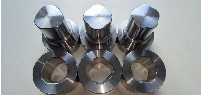
Figure 5. Epitrochoidal inner and outer contours for shaft–hub connections produced using the twin-spindle process; source: Iprotec:Guido Kochsiek [12].
