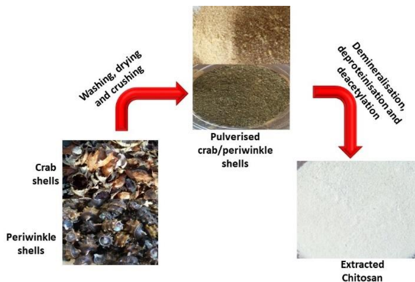
Figure 2. A simplified scheme for chitosan extraction from crustacean shells.
