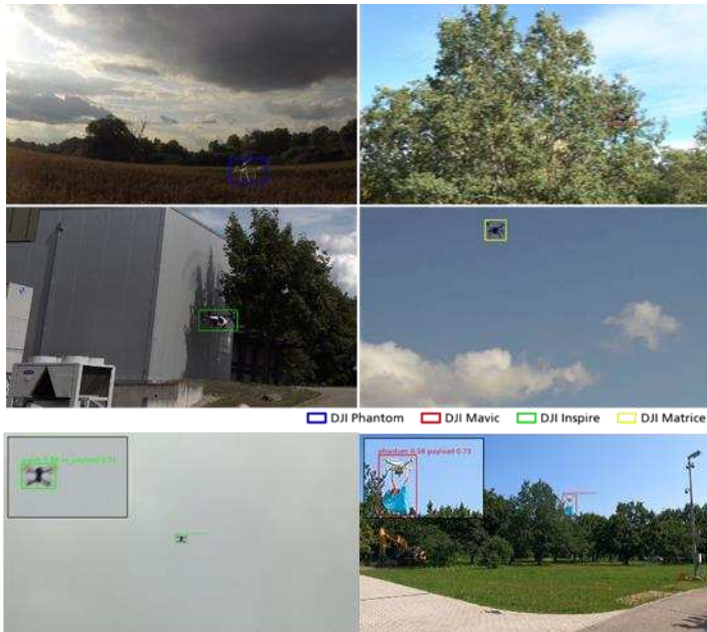
Figure 5. UAV classification by model (top) and payload (bottom).
