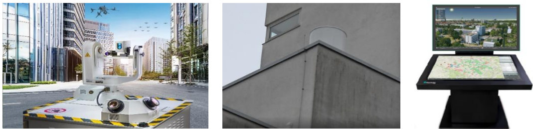
Figure 1. MODEAS: optical sensor station (left), radar station (middle), and control center (right).
