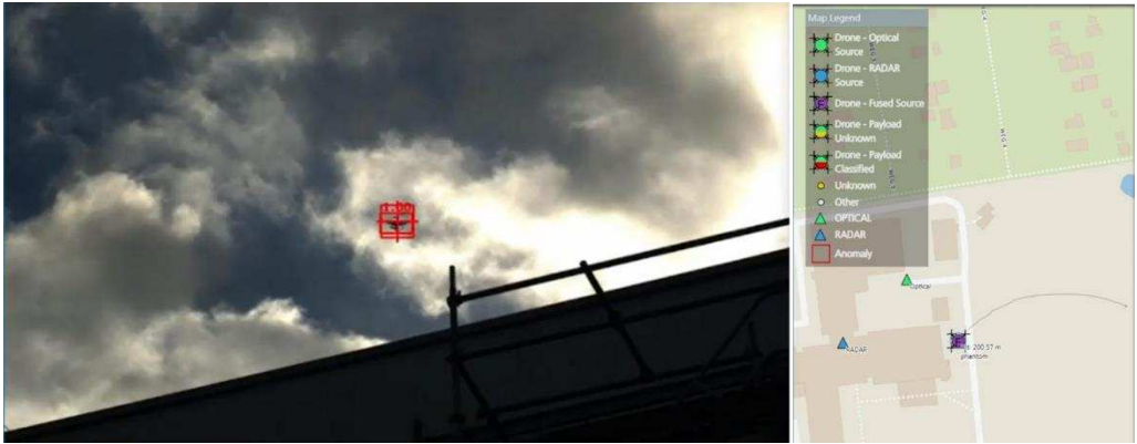
Figure 10. Visualization of a fused detection of both radar and optical sensors on the Digital Map Table.
