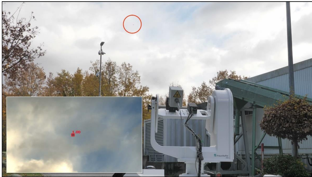
Figure 9. Detect and track a drone with the PTU-camera.
