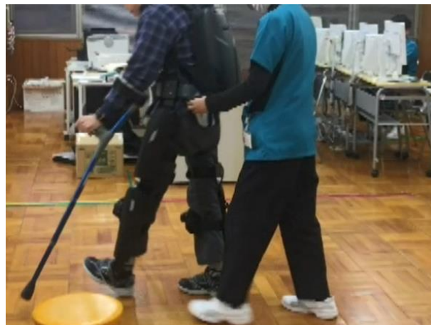
Figure 1. Gait rehabilitation using a powered exoskeleton in a patient with spinal cord injury. A physical therapist is seen behind the patient to provide gait balance adjustment and contact assistance to prevent falls.
