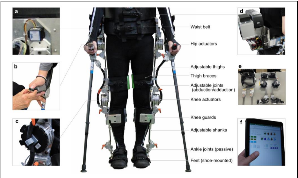
Figure 2. Appearance of the prototype powered exoskeleton for spinal cord injury. (a) Gait trigger sensor. (b) User interface with a remote control built into Lofstrand crutches. (c) Actuators attached to the hip and knee joints. (d) Control unit and battery. (e) Separable frame. (f) Adjustment software installed on a Tablet PC.
