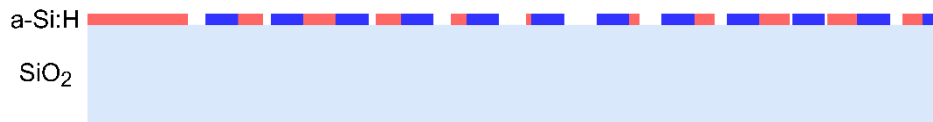
Figure 15. Grating coupler made from the superposition of two diffraction gratings with periods of 1500 nm (represented in red) and 1300nm (represented in blue), the result is a grating with a chaotic (random) distribution.
