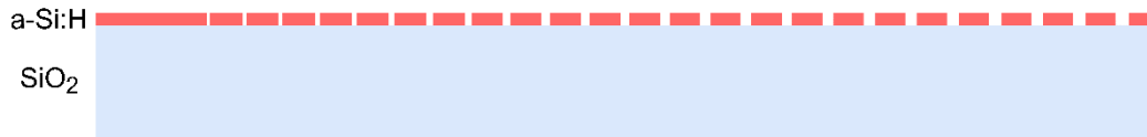
Figure 12. Grating coupler with a quadratic variation of the refractive index, fill factor and period vary over the grating's length. The refractive index is the highest close to the waveguide (at left) and the lowest at the end of the grating coupler (at right). Only 24 segments are represented. Representation accurate to 1/100th of a micrometer ( \pm 10 nm tolerance per segment).
