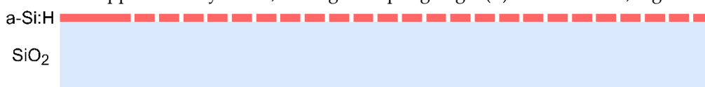
Figure 13. Grating coupler with a period of 690 nm and a fill factor of 82.6 %. First 24 periods represented, coupling angle not represented.
