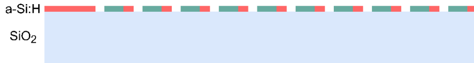
Figure 14. Grating coupler made from the superposition of two diffraction gratings with a period of 1500 nm, the result is a grating with the same period and a fill factor of 76.6%.
