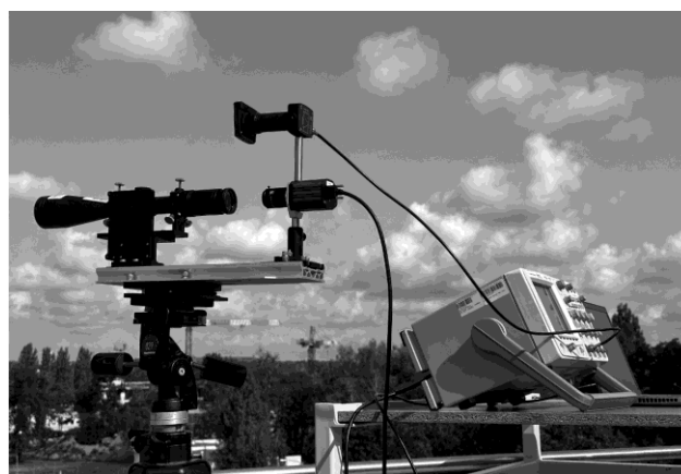
Figure 7. Measuring device: Si Avalanche Photodiode with a UV filter (upper) with visible sight camera (lower).
