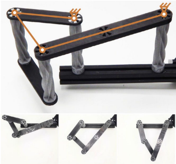
Figure 41. A neutral and stable four-bar linkage mechanism (orange schematic) consists of a rigid linkage (black) and a helical shell joint (gray). These joints are preloaded to move within a constant torque range. At the bottom, top views of some equilibrium positions are displayed [103].
