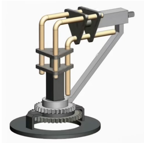
Figure 84. Schematic diagram of right-angle transmission mechanism [150].
