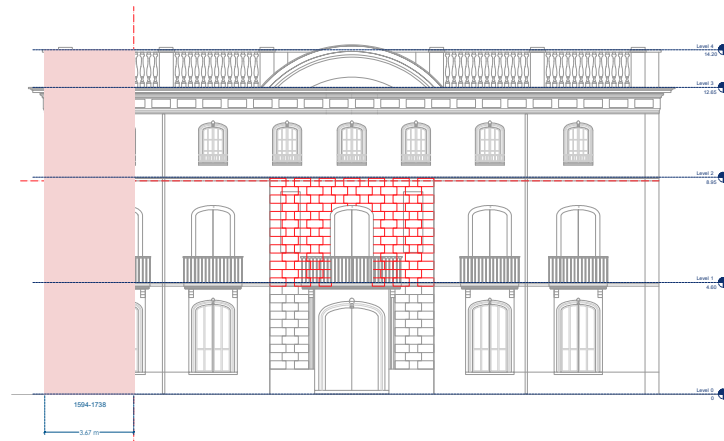
Figure 28. Drawn south façade anomalies.
