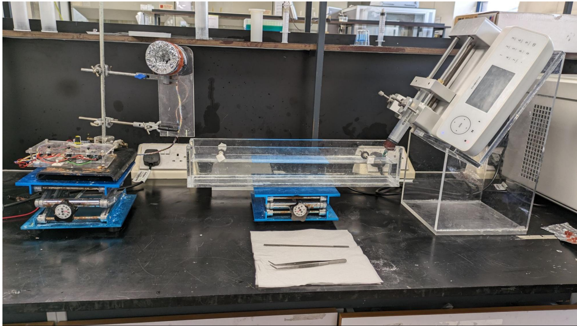
Figure 7. Wet spinning device developed in the [Anonymised University Name for review].
